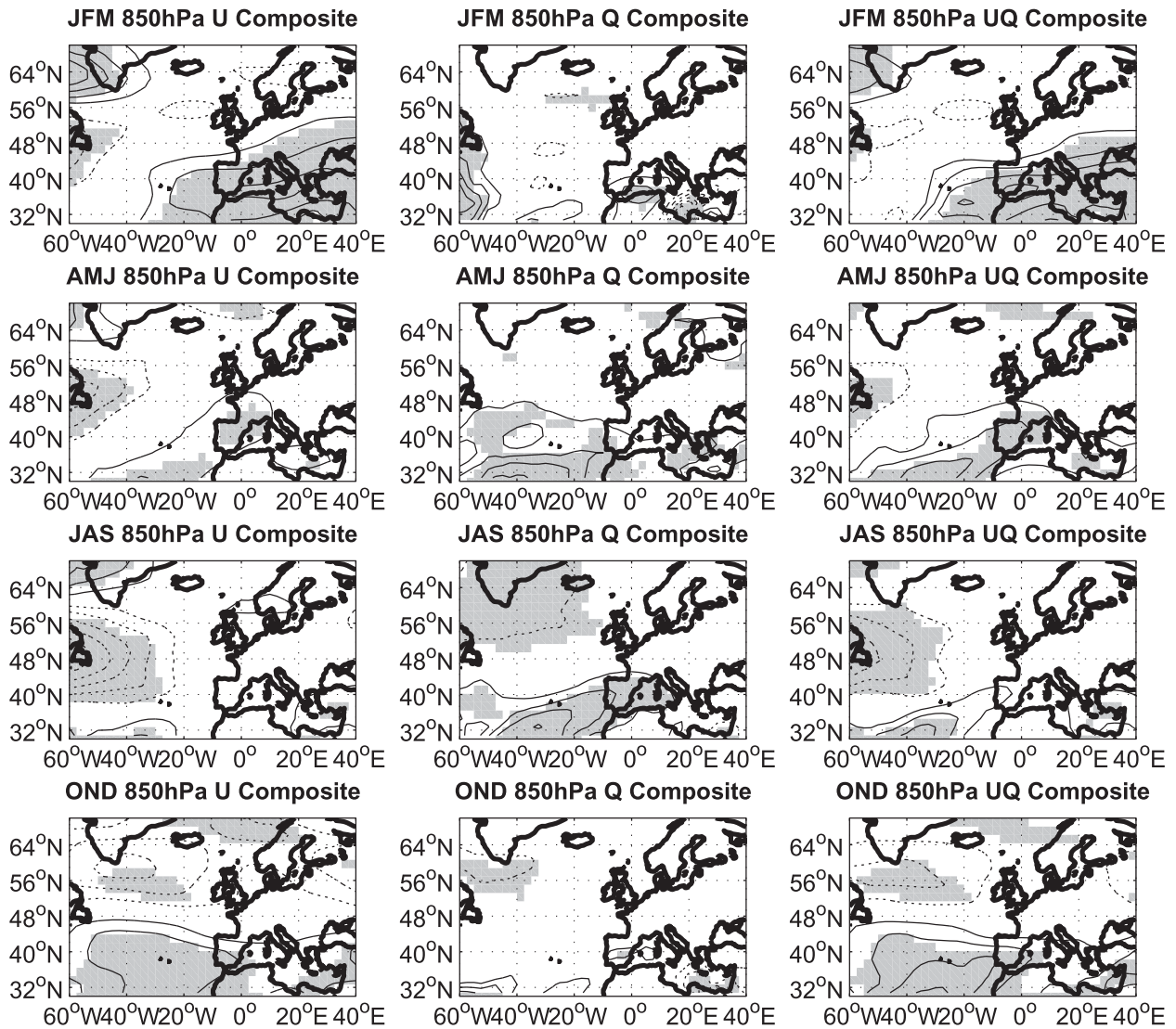
FIG. 12. The 3-month seasonal ENSO-based composites of 850-hPa (left) zonal wind, (center) specific humidity, and (right) zonal humidity flux derived from an 1870–1999 integration of CAM4. The contour intervals are (left) 0.5 \text{ m s}^{-1} , (center) 1 \times 10^{-4} \text{ kg kg}^{-1} , and (right) 2 \times 10^{-3} \text{ kg kg}^{-1} \text{ m s}^{-1} . Negative contours are dotted and the zero contour is omitted. Gray areas denote regions significant at the 95% level ( p < 0.05 ) based on bootstrap confidence intervals estimated by generation of 5000 random CAM4 composite maps for each 3-month seasonal period.
