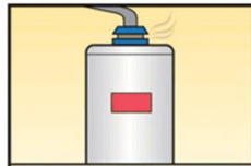
Corroded or Disconnected Water Heater Vent Pipe
