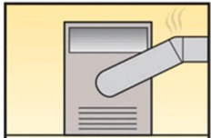
Cracked or Loose Furnace Exchanger
